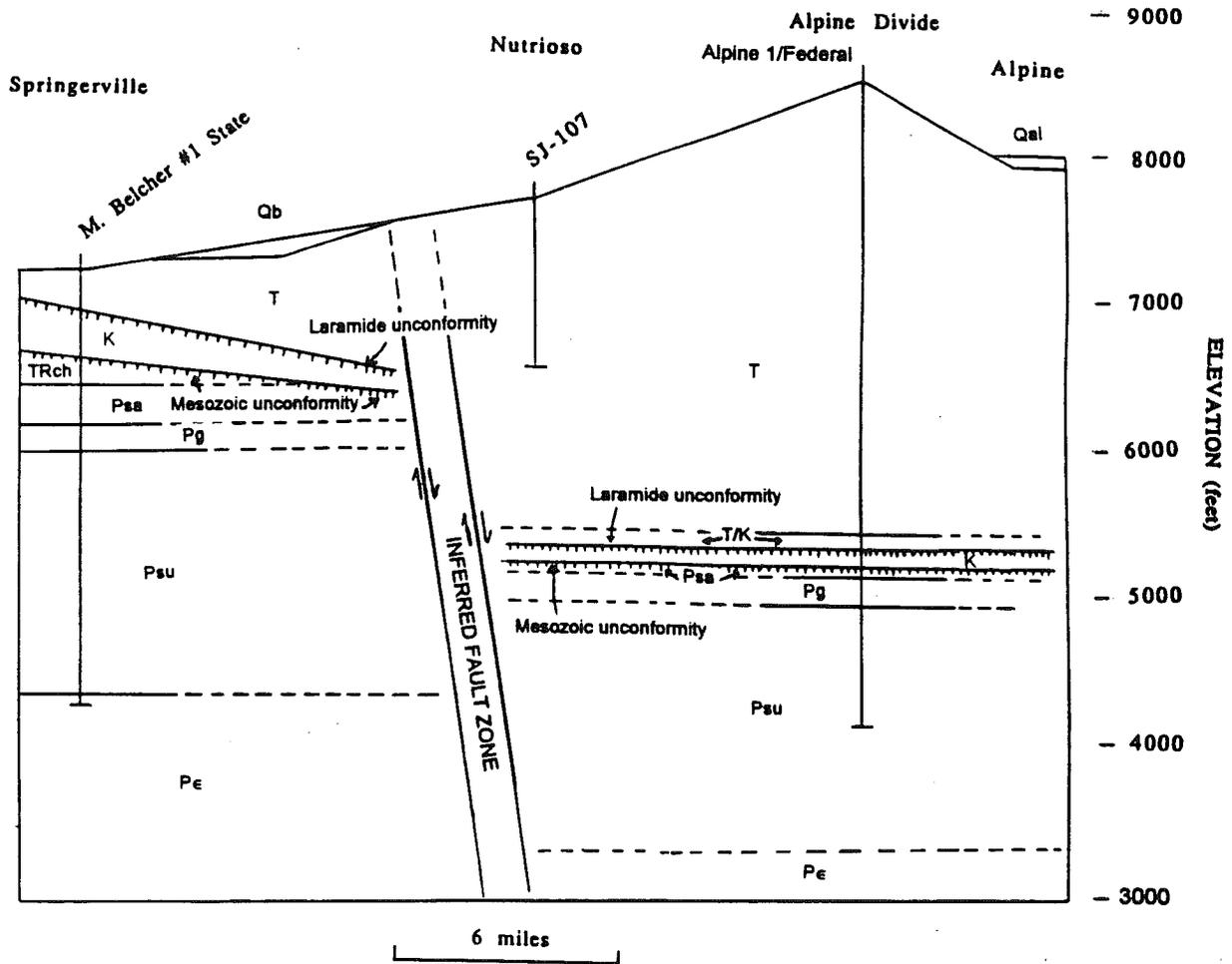
Figure 5. Post-drilling geologic model of subsurface geology.
