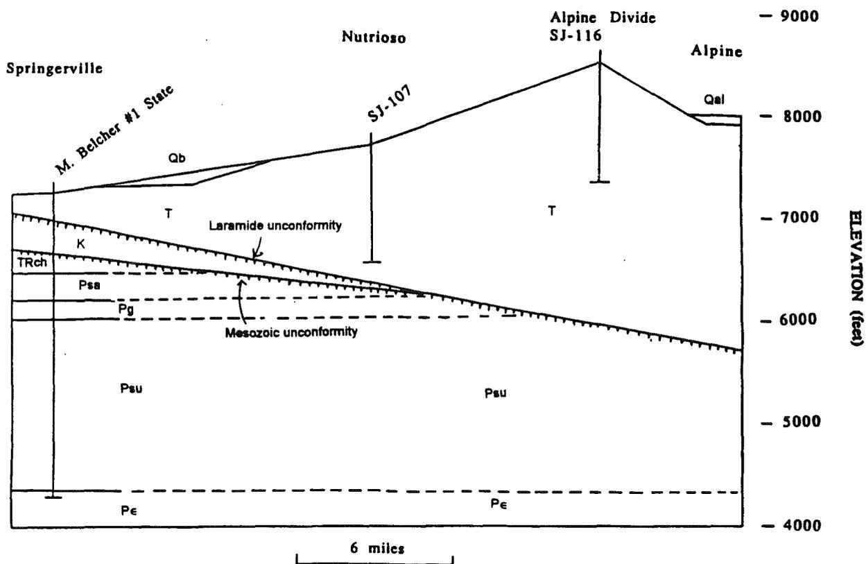
Figure 4. Pre-drilling geologic model of subsurface geology.
