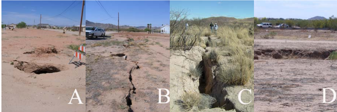
Figure 1. Earth fissure surface expressions are classified into four categories A) circular depressions “potholes”, B) surface cracks, C) gullies, and D) displacement.
